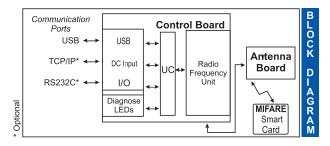
The *MicroSMART* USB Proximity Reader (Short Range) consists of a MIFARE RC 632 Smart IC, a ARM CPU and a USB interface mounted on a PCB. It also carries the antenna for the data communication with a contactless MIFARE compatible Smart Card. It can optionally be provided with TCP/IP LAN Port for Network based application. It can acts as a Wiegand Reader also.
